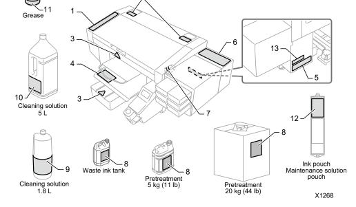
This printer has the following warning labels displayed on it. Follow the precautions given on each warning label for your work.
