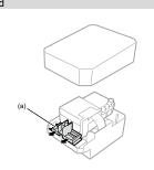
When you unpack the head, be careful not to touch the bottom of the head. Otherwise it may cause poor printing When you mount the head, shift the carriage toward the center of the printer; to the position above the platen. If you perform the mounting of the head when the carriage is directly above the maintenance unit, it may damage the maintenance unit or the heads.
