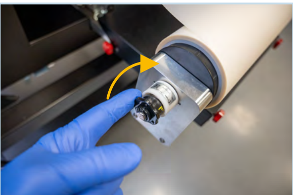
Then slightly, with one finger, turn each knob clockwise till you feel a slight resistance. It is best to set the buttons identically.
