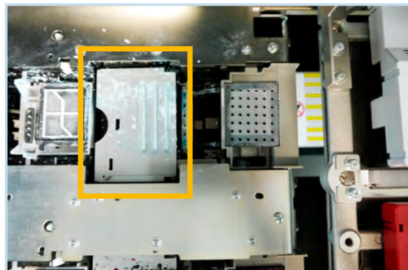
Position of the wiper cleaner (white side).
