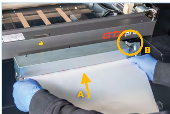
A: Insert the film carefully and in an even way. B: The lock lever must be down to be open.
