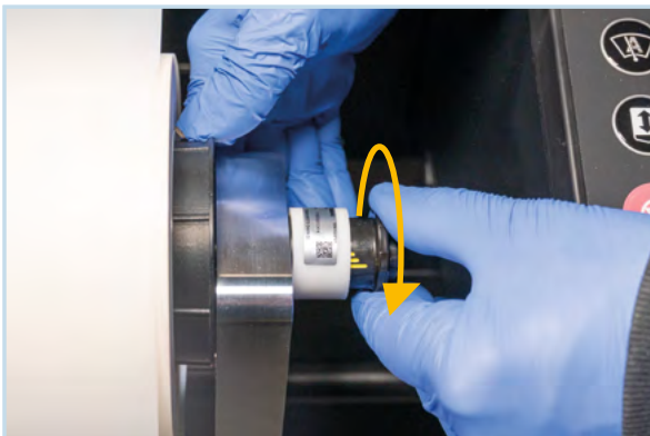
Turn the brake knob right side counter-clockwise until it stops to release the brake completely.
