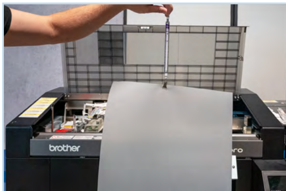
HELPFUL: Attach a spring balance to the film and slowly unroll it a little. The resistance value should not exceed 100 gr.
