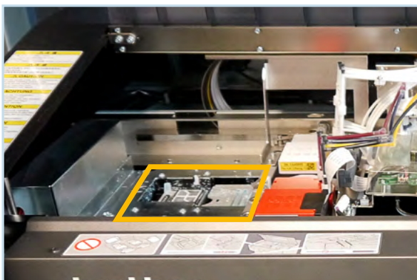
Position of the cappings, exhausts and wipers.
