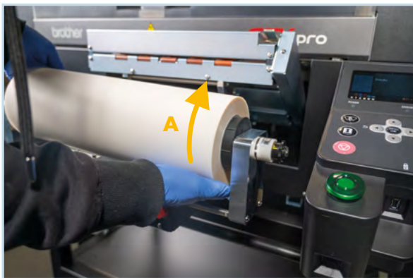
Insert the film roll between the jaws. A: The rolling direction
