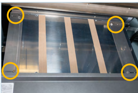
Align the film straight on the print table. If you use a 40cm roll, remove the screws from the side guides and screw them back into the outer holes.
