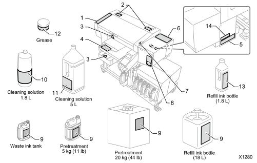
This printer has the following warning labels displayed on it. Follow the precautions given on each warning label for your work. When the label is peeled off or illegible, contact the place of purchase.
