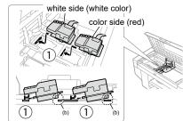
Insert the head firmly to direction (1).
