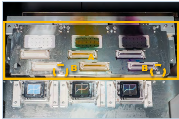
A: Clean the Shield Plate with a Cleaning Stick R B: Check that the two hooks are snapped in
