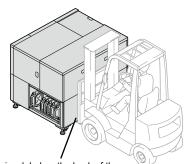
There is a label on the back of the printer that indicates the insertion slot.
