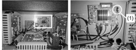
2) Remove the Lithium Battery (1) by pulling out the holder in the direction of the arrow.
