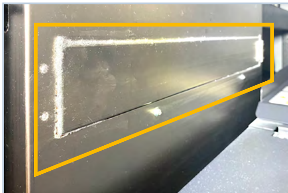
Clean the doors of the Mist Fan Filter and the surrounding area
