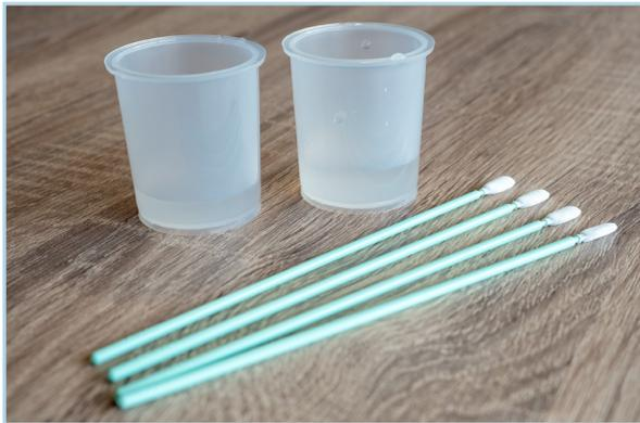
Fill two Cleaning Cups with 10 - 20 ml of fresh Cleaning Solution. Prepare 4 Cleaning Sticks T.
