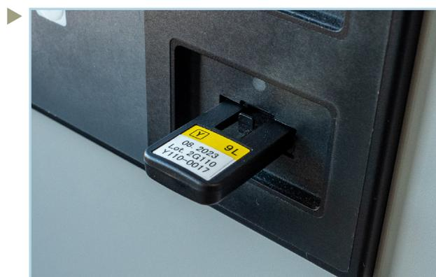
Insert the IC-Stick of the liquid you want to refill and press OK.
