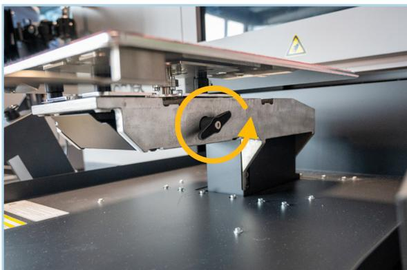
Turn the knob under the platen counter-clockwise.
