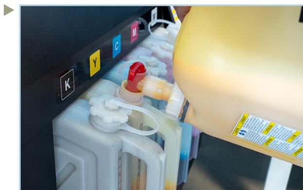
Refill the ink or cleaning solution. Make sure to not exceed the line above the 6 mark.
