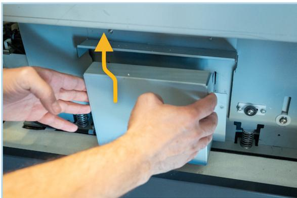
Remove the CAM cover by lifting it a little and then pulling it out.
