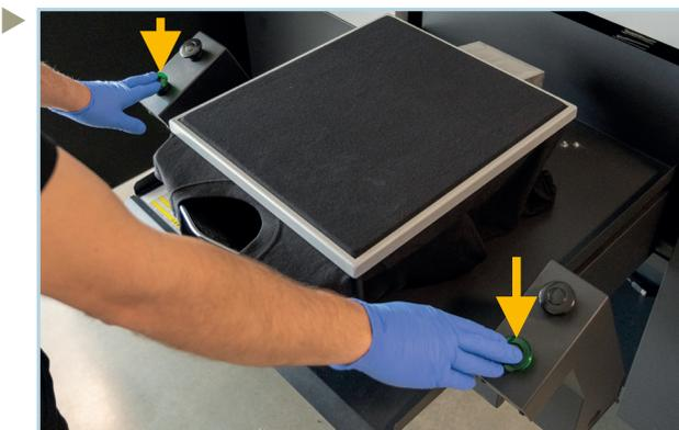
When the (pretreated) garment has been mounted on the plate and the printfile has been loaded, the print is started by pressing the two green buttons simultaneously.
