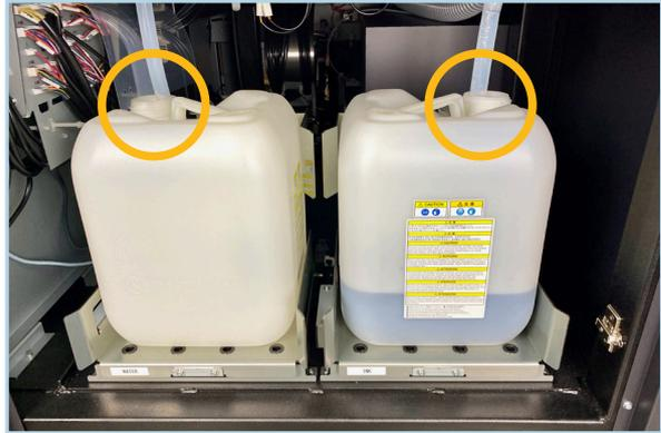
Detach the tube of the tank you want to empty. Be careful to not create splashes with the waste ink tube.
