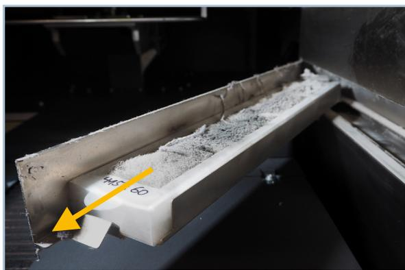
Remove the Filter and clean the compartment.
