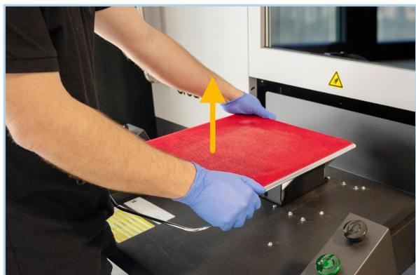
Lift the platen straight up. Store the platen in a safe place.
