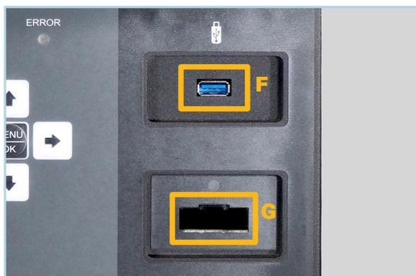
F: USB 3.0 port Type A to load print files from an USB-stick.
