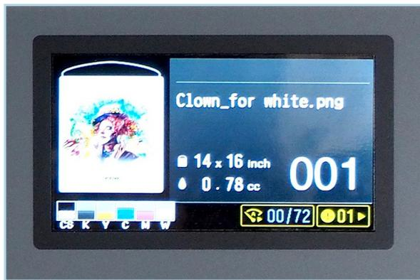
The display shows the current loaded print file with the used platen and the approximate ink consumption.
