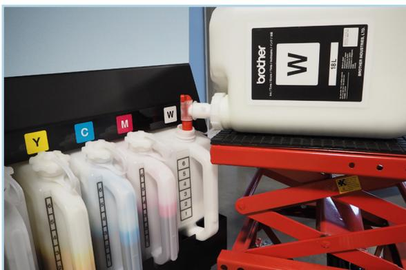
It is recommended to use a hydraulic scissor lift and the enclosed faucet to refill the white ink.
