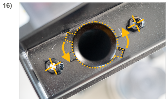
Turn the bracket until the nuts are aligned to the holes on the column.
