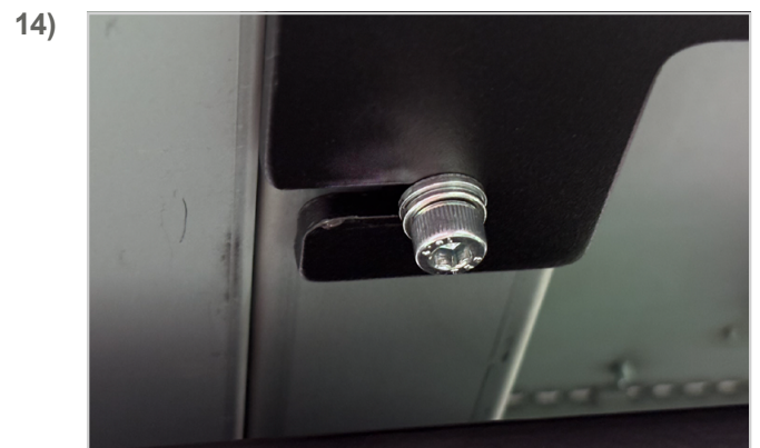
Tighten the rear screw.
