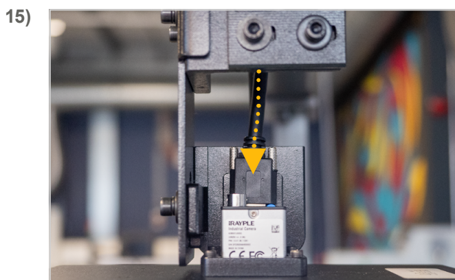
Connect the camera data cable to the camera. Then connect the data cable to your PC.
