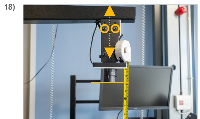
Set the printer platen to height B. The distance between lens and platen should be 657 mm. The tolerance is \pm 5 mm.
